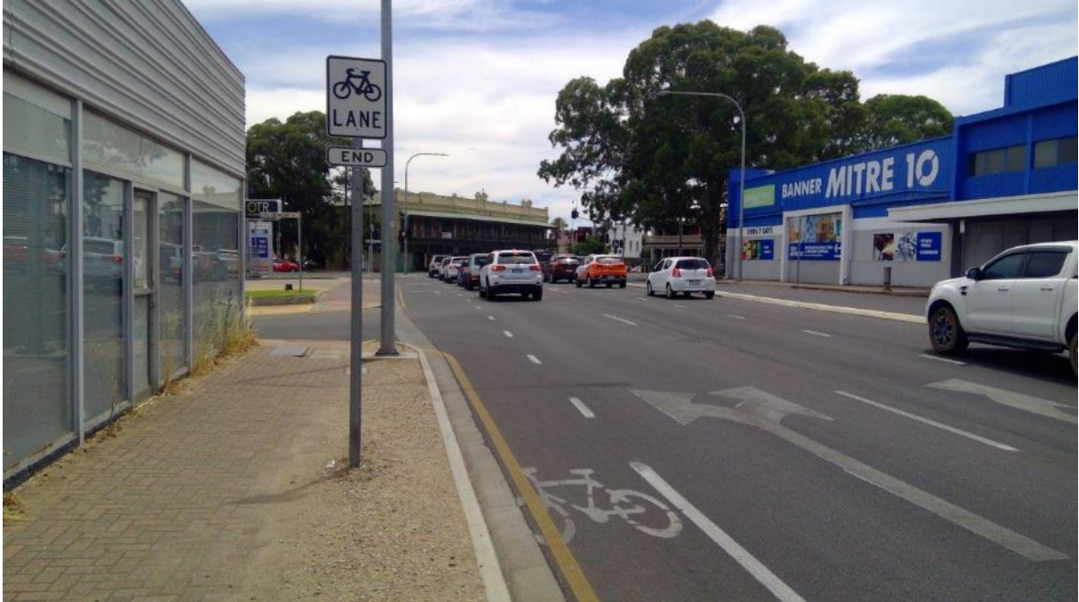
Figure 36: The northbound cycle lane ends to make way for a turn lane on approach to Payneham Road
